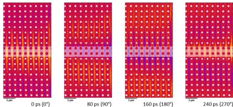
Figure 1: Dynamic X-ray micrographs with magnetic contrast (XMCD) at different time steps of a movie showing the propagation of a spin wave mode in an antidot lattice. The spin wave can only propagate between antidots. The applied external bias field allows propagation over 10  $\mu\text{m}$  from the excitation source. The positions of the stripline and the antidots are indicated as white overlays.
