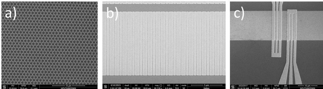
Scanning electron microscopy images of: a) \text{Ni}_{80}\text{Fe}_{20} kagome lattice, b) quasiperiodic \text{Ni}_{80}\text{Fe}_{20} stripes and c) CoFeB/NiO microstripe with deposited CPWs
